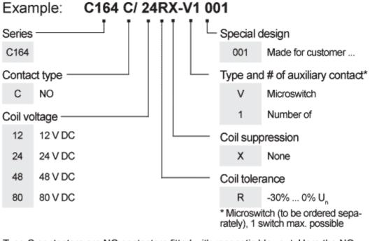
Type C contactors are NO contactors fitted with magnetic blowout. Here the NO contact functions as circuit-breaker within an open contact design. Type I contactors, however, feature an additional NC contact which is galvanically isolated and has a potential of its own. So, for type I SPDT contactors is to be observed that only the NO contact may be used for breaking the circuit, whereas the NC contact should only be used for power transmission functions.
